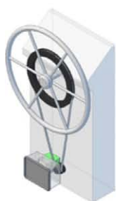
Horizontal Motor Box 2 ¼" (57mm) minimum distance from spokes to bulkhead
